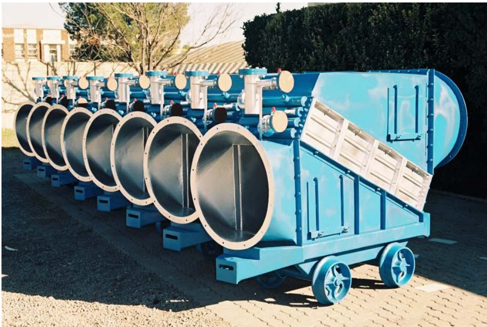
100kW Trojan Cooling Coil Cars
