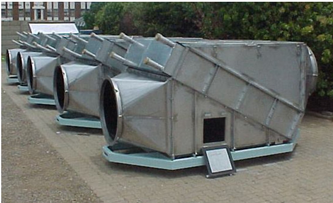
420 kW Cooling Cars with top-hinged inspection cover.
