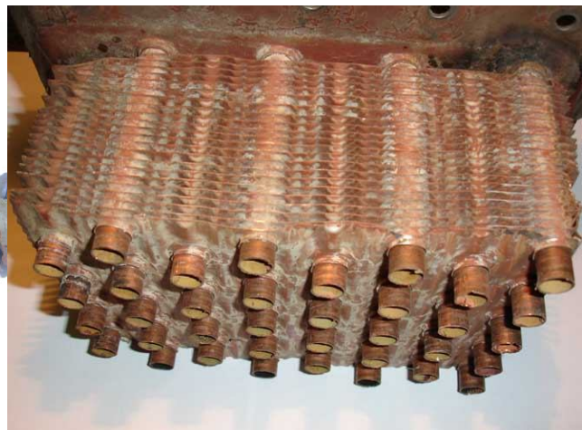
Plate fin type coil with copper tubes and aluminium fins.
