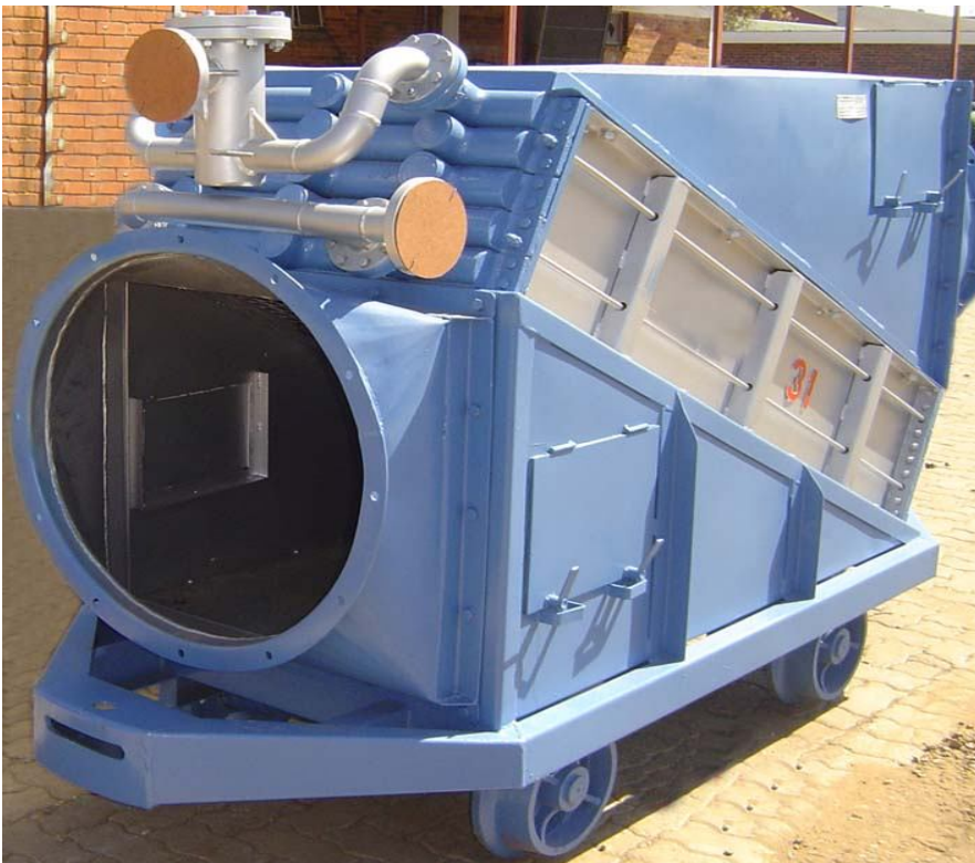
New 300 kW Cooling Coil Car with 316 s/s headers and HIFIN tubes.
